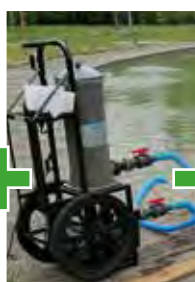
EXTERNAL PUMP ON ITS TROLLEY
